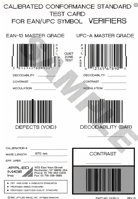
Figure 3 : Verifier Conformance Calibrated Test Card
