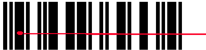
Figure 11 : Example of too small aperture size
