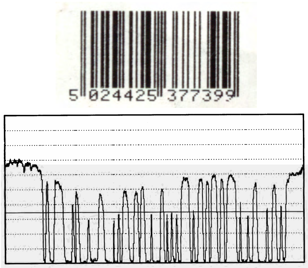
Figure 20 : Symbol with "edge determination" problem and associated Scan Reflectance Profile showing narrow space profiles failing to reach Global Threshold, giving Decode failure
