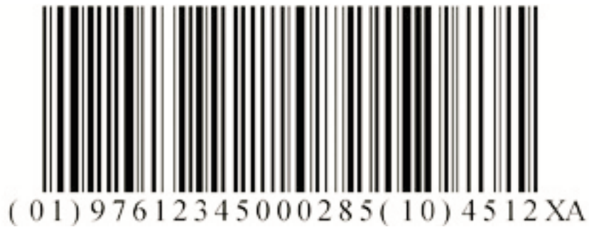
Figure 7 - Example of UCC/EAN-128 bar code
