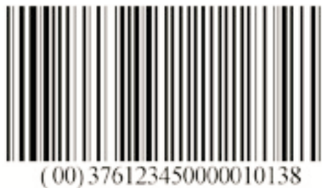
Figure 9 – Homogenous logistics unit bar code example
